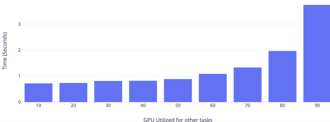
Fig. 8. Average Runtime at each GPU utilization percentage
